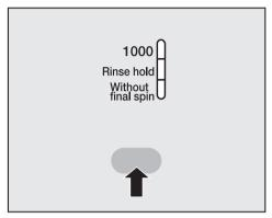
Press the "Spin" button repeatedly until the indicator light for the required selection lights up.
